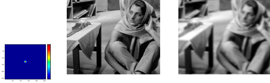
Figure 2. Image deblurring problem: (LEFT) Point Spread Function; (CENTER) Exact image; (RIGHT) Blurred image.
