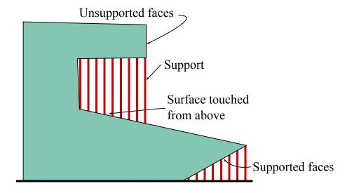
Figure 3.3.2: In this vertical cut of a 3D object, we can see that the surface can be divided in three parts. *Unsupported faces*: parts of object that do not need external support to print; *supported faces*: parts of object that need external support underneath them to print; and *support faces*: parts of object that are touched from above by the support structure. This figure was created based on figures in (ALEXANDER; ALLEN; DUTTA, 1998).
