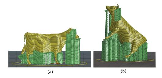
Figure 3.2.3: Surface *cow.obj* at the initial vertex position (a) and after rotation (b) minimizing the objective function 3.1.3. Even getting less overhanging parts, this objective function does not consider the surface area and height of support, which, in this case, causes the amount of support to be larger than desired.
