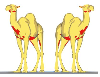
Figure 3.0.1: Camel surface from Libigl (JACOBSON et al., 2018) in the initial position (left) and after  $\theta = \frac{\pi}{3} z$ -axis rotation (right). The red area of both surfaces are those that need support to print. Notice that the support area does not change after this z - axis rotation.
