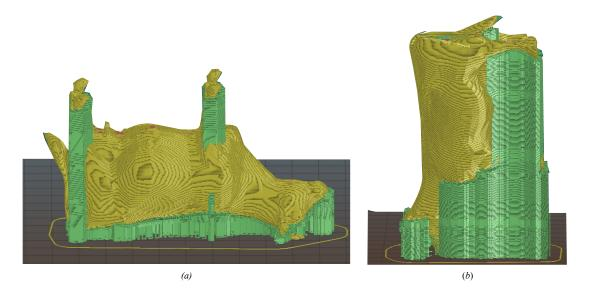
Figure 3.4.4: Libigl surface *cow.obj* after rotation using our method (a) and Alexander's method (b). As we can see, these results using our method generate less support for overhanging parts of surface then Alexander's method.
