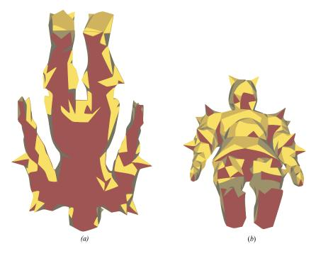
Figure 3.4.5: *decimated-knight.obj* surface after rotation using our method (a) and Alexander's method (b). As we can be seen, the result using our method generates more overhanging parts area (in brown) than Alexander's method.
