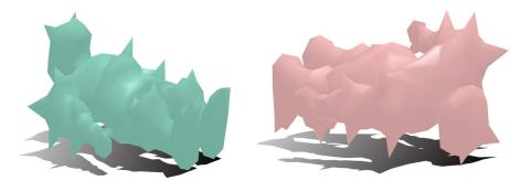
Figure 4.2.2: Knight surface from Libigl (JACOBSON et al., 2018) after global rotation on tests performed on section 3.4 (left) and after finding a local minimum using *fmincon* Matlab function with a chosen initial point (right). The teal surface on the left would be printed in 136 minutes with 3g of material loss (support that would be wasted) and the pink surface on the right would be printed in 149 minutes with 5g of material loss.
