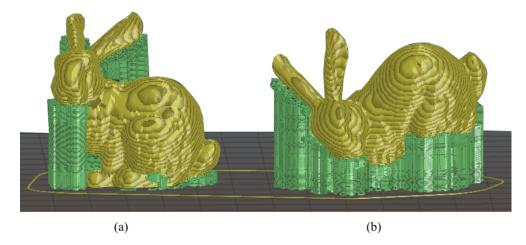
Figure 3.1.9: Surface *Bunny.obj* at the initial vertex position (a) and after rotation (b). In yellow, the software indicates the solid that we want to print and in green the overhang supports. With Slic3r sorftare we can observe that the objective function 3.1.3 returns an orientation of this object with more support than initial position.
