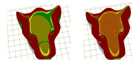
Figure 3.1.2: Lion surface from Libigl (JACOBSON et al., 2018) with 0% infill (left) and 30% infill(right). The parts of the surface such that normal angles are above the support angle threshold  $\theta$  will also need some support to be printed, if the printer infill is set to 0%.
