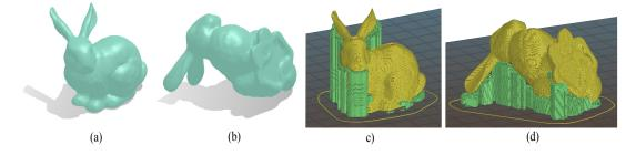
Figure 3.4.3: Libigl surface *bunny.obj* on the initial position (a) and after rotation (b). On 3D print sorftware (Sklic3r), the same surface on the initial position (c) and after rotation (d). Also, in figures (c) and (d), the software indicates the surface in yellow and the overhang supports in green.
