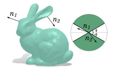
Figure 3.1.1: This two normals  $n_1$  and  $n_2$  of the bunny surface have different angles. The normal vector  $n_1$  is within the angle range of the printer. The normal vector  $n_2$  is in an overhanging part and will need a support to print correctly.
