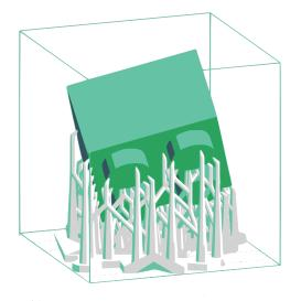
Figure 1.1.2: This solid has parts that need support to print correctly. So the printer will build some structures to hold this parts while it is printed.
