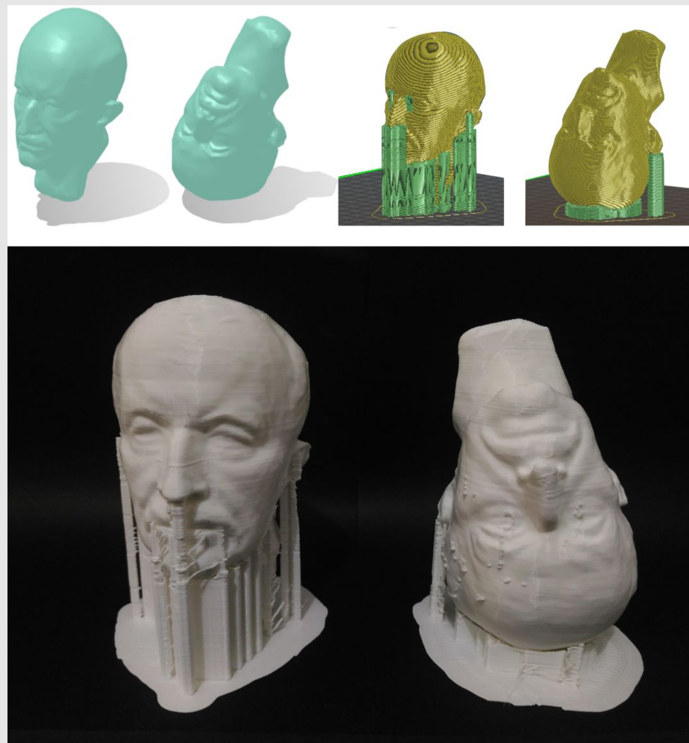
Fig. 5 - Face.obj on the initial vertex position (top-left) and after rotation (top-center-left). The same surface on the initial position on the print simulator (top-center-right) and after rotation (top-right). In yellow, the software indicates the solid that we want to print and in green the overhang supports. The bottom figure is a photo of same surface after printed. On the bottom-left, the surface is on the initial vertex position and on the bottom-right, the surface is positioned after rotation procedure.
